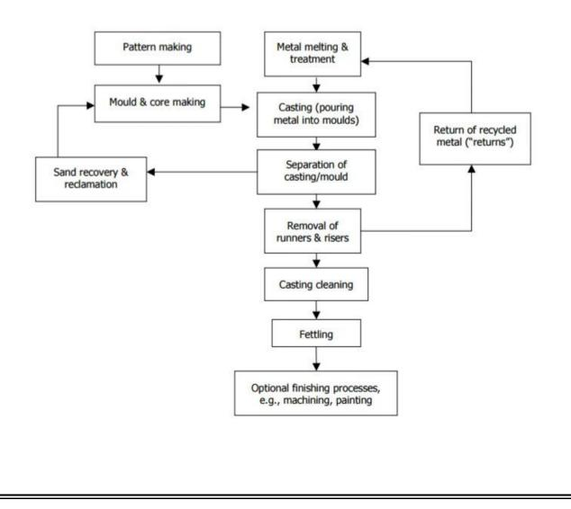
Description of the foundry process Foundries produce castings that are close to the final product shape, i.e., "near-net shape" components. Castings are produced by pouring molten metal into moulds, with cores used to create hollow internal sections. After the metal has cooled sufficiently, the casting is separated from the mould and undergoes cleaning and finishing techniques as appropriate.
