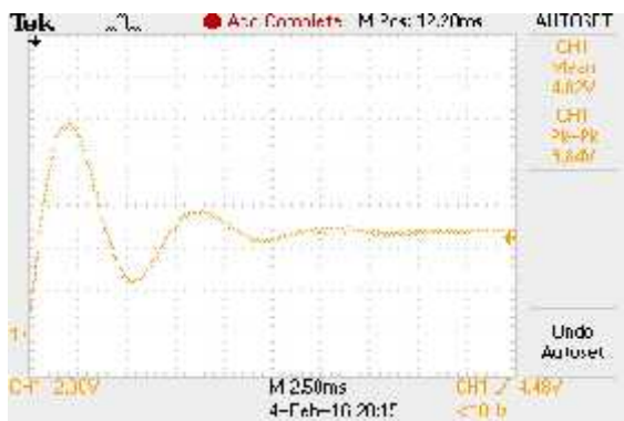
Fig.h. Real-Time simulation result- Inductor current vs Time, scale- 1:1
