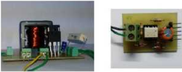
Figure 10 Buck Converter and Gate Drive Card
