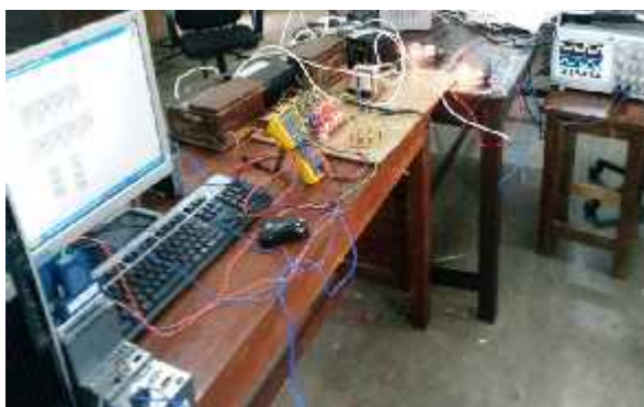
Fig. 3. Experimental prototype of the dual input DC-DC converter
