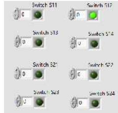
Fig. 6. Fault indication for fault in switch 'S12'.
